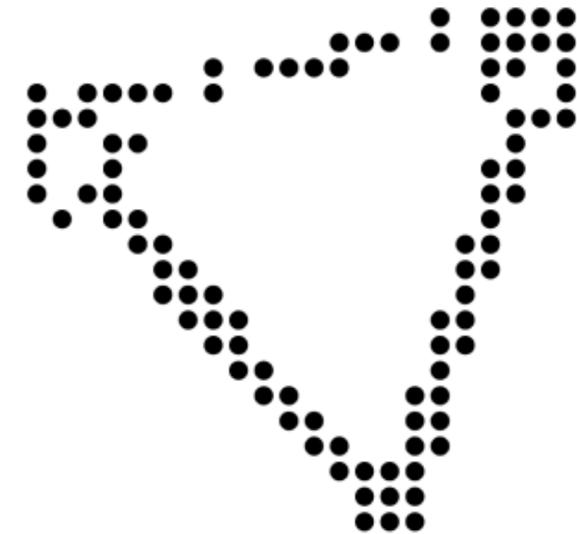
C. Braille pin array output
